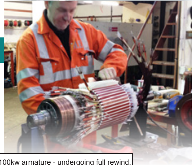
100kw armature - undergoing full rewind. This is being wound as a spare for a polythene extruding company
